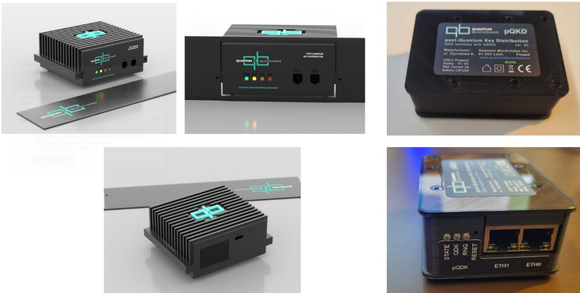
Figure 7. pQKD devices: design of the final product (left), the functioning prototype (right).
