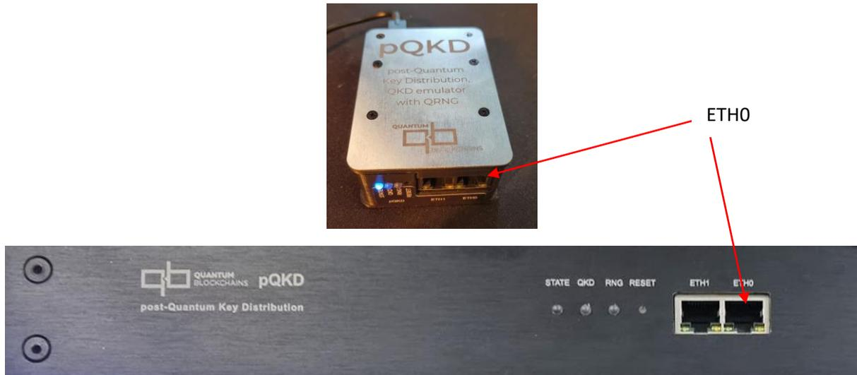
Figure 21. Desktop and Rack Mounted pQKD. Use the rightmost (ETH0) LAN RJ-45 connector.
